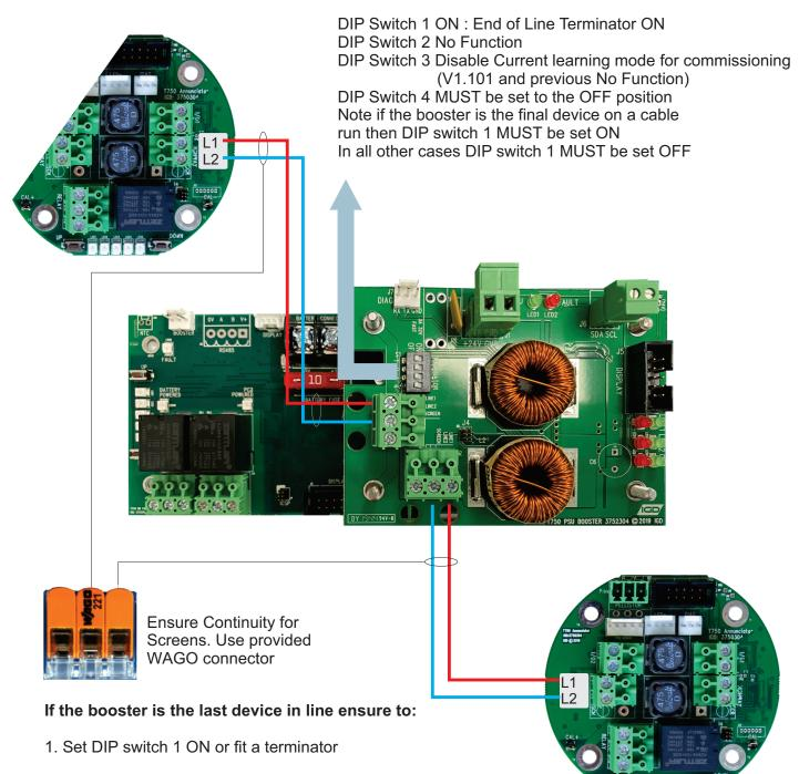
2. DO NOT ground the cable screen in the booster module ONLY ground the screen at the control panel.
