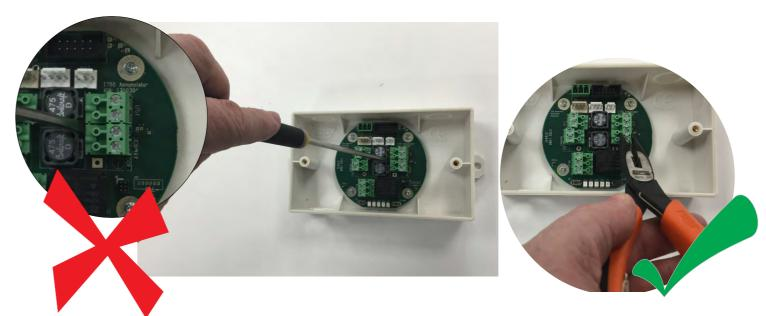
When unplugging detectors from the main PCB DO NOT lever them off. This will potentially cause damage to the PCB and/or connector mating parts and invalidate any warranty. If it is necessary to remove the PCB connectors use long nose pliers.
