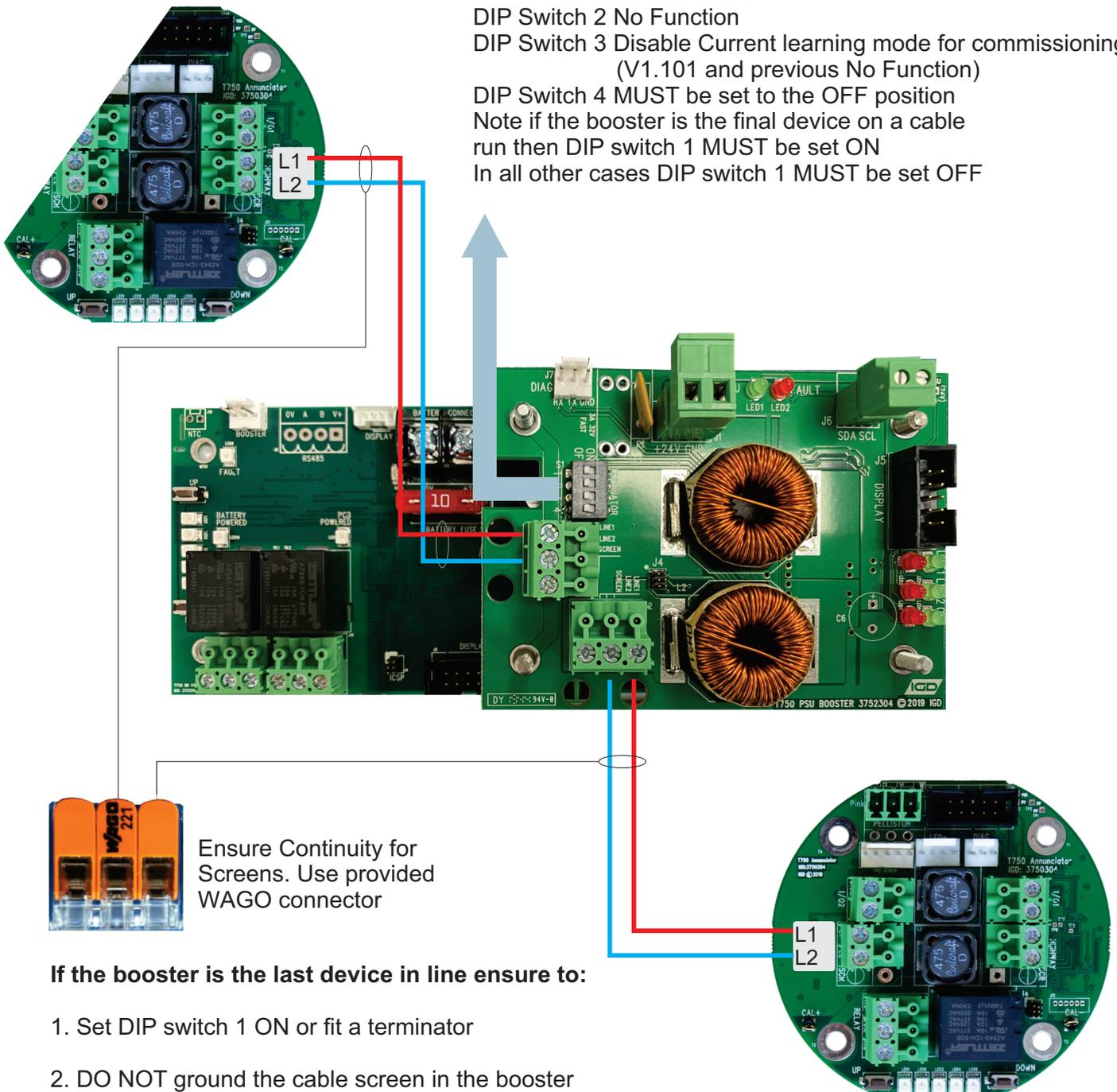
If the booster is the last device in line ensure to:
