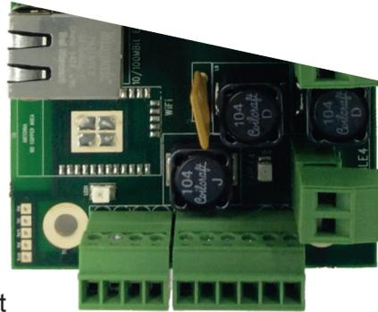
Power Connections to 650/750 Control Panel. Note This is a 4 Core Cable to Share Load and as a Minimum 1.5mmSQ Cable as Short as Possible
