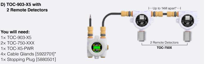
\*Cable glands don't come with the TOC-750X, example shown is for 2 detectors \*\*TOC-X5-TERM (Terminator) one is required per end of line
