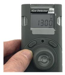
**STEP SEVEN** Check the charge level and if necessary charge the unit using the charger and cable supplied.
