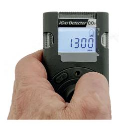
**STEP EIGHT** Press the right hand button to bring on the backlight for a short period when reading in low light levels.
