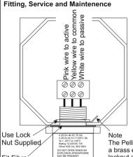
Head operating current should be adjusted to 360mA +/-2mA. Pellistors should be allowed to stabilise for a minimum of 2 hours on initial connection prior to calibration. Only connect to approved IGD bridge circuits. If in doubt check compatability with Oliver IGD Limited
