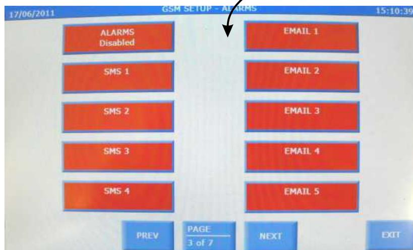
Set up page 3 allows you to determine what is sent to each email or SMS number. The button tops will stay red until a set up is configured for each address or number. selecting the button for a particular address or email account allows you to cycle through options on each button press.
