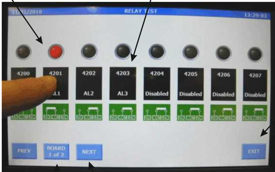
Use EXIT to return to the main menu and release all selected relays back to normal operation.
