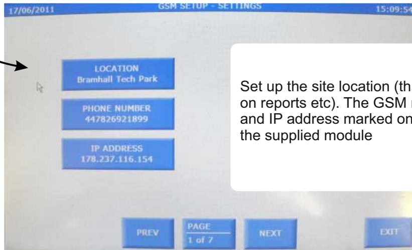
Set up the site location (this appears on reports etc). The GSM number and IP address marked on the supplied module
