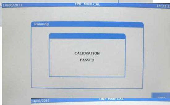
Sensor has passed calibration. The system will now wait for gas to be applied to the next sensor.
