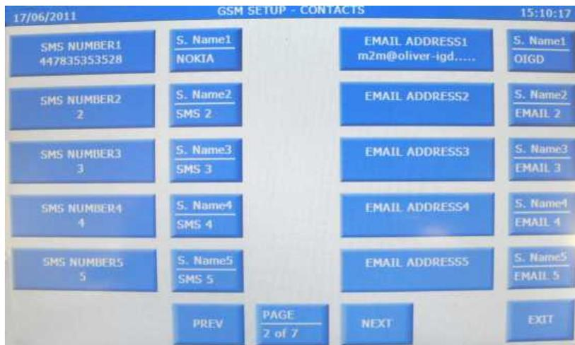
In set up page 2 you can set up to 5 telephone numbers for SMS alerts and 5 email addresses. Once set up these will receive any alarm or status reports requested or sent from the system.
