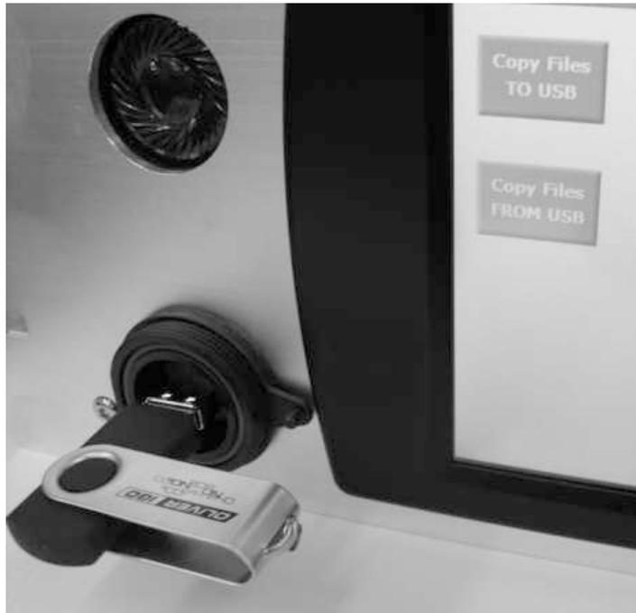
Ensure the pen drive is fitted to the USB port.
