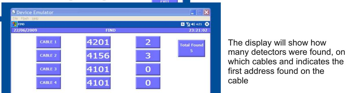
The display will show how many detectors were found, on which cables and indicates the first address found on the cable
