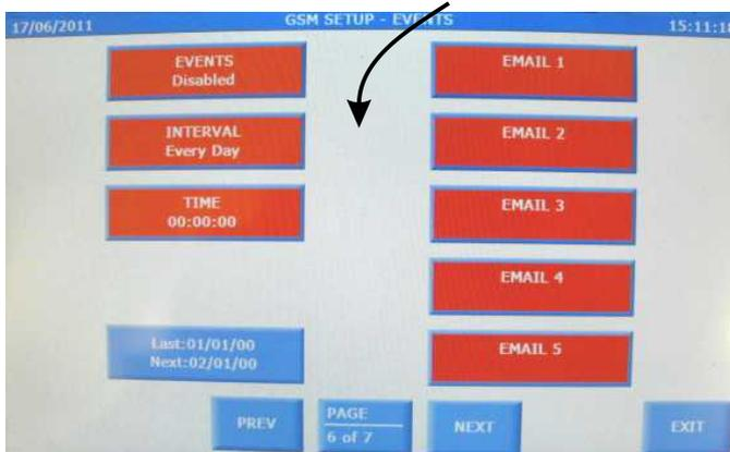
Page 6 of the GSM set up determines for the Events report the frequency it is run at and which email address gets the automated report at the interval set.
