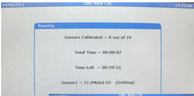
First sensor has had gas applied and is into the settling period. Time left is displayed. If gas is not applied to a sensor for more than 60 minutes then the sequence times out and the system returns to normal operation
