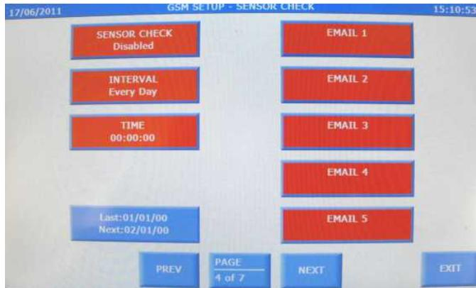
Page 4 of the GSM set up determines for the system sensor check report the frequency it is run at and which email address gets the automated report at the interval set.
