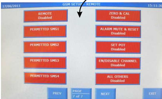
Set up page 7 determines for the mobile phone numbers configured, which ones can access which remote command features.
