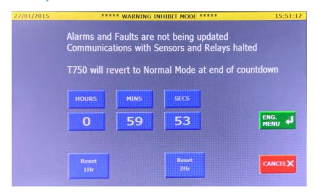
Entering Pass Code 25 will place the system into inhibit mode. Initially this will be for 60 minutes and can be terminated by selecting cancel at any time. During inhibit mode the system is not communicating to its detectors and so will not respond to them. Typically inhibit mode is used during system maintenance when Android/tablet IGD service tools are being used.
