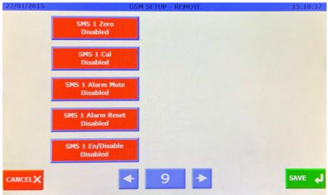
Screen 9 allows selection to enable selected SMS users interaction with the system.
