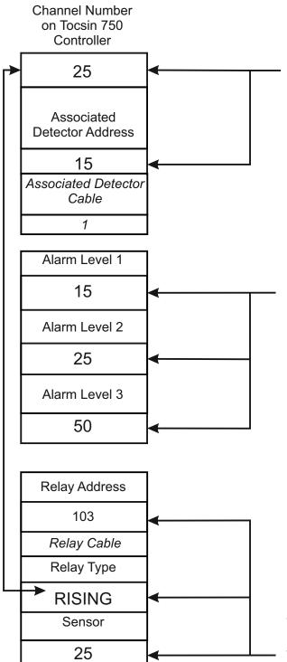
In this example for this particular channel (25) on the Tocsin 750 controller the gas detection readings are coming from detector 15. This is setup in the SENSOR SETUP menu.
