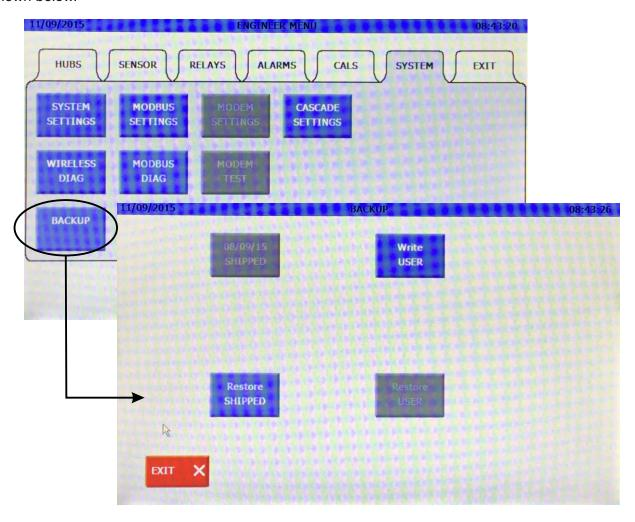
If the controller was shipped with a factory configured alarm setup then the 'as shipped' backup will already be saved. This is indicated in the screen display shown above. This setup can then be restored at any point by selecting 'Restore Shipped'.
