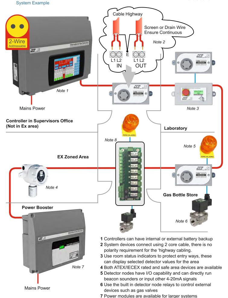
8 Fit i/o cards on the same highway where control is required
