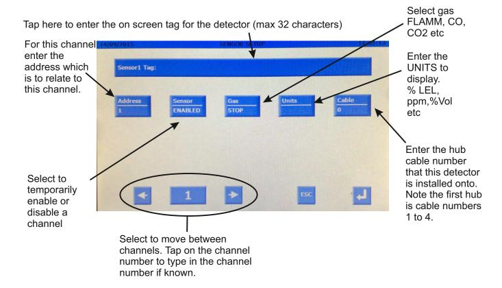
Note that when a set up button is selected a popup menu appears to allow data to be typed into the set up box.
