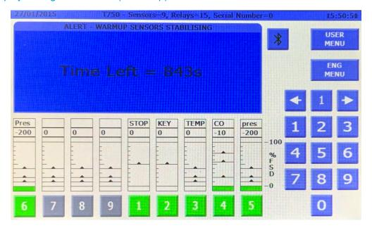
On initial power up the system will run a series of system checks and then start a stabilisation 'warm up' timer. For systems including Oxygen sensors this will be 15 minutes, other sensor types 5 minutes. During warm up alarm relays will be in their 'normal' non-alarm states. A modbus state is available to indicate warm up status.
