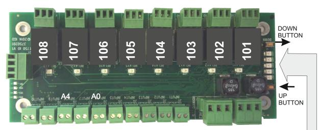
Press and hold the DOWN button until all LED's are OFF. Release the button and the address currently set will be illuminated on the bottom five LED's.
