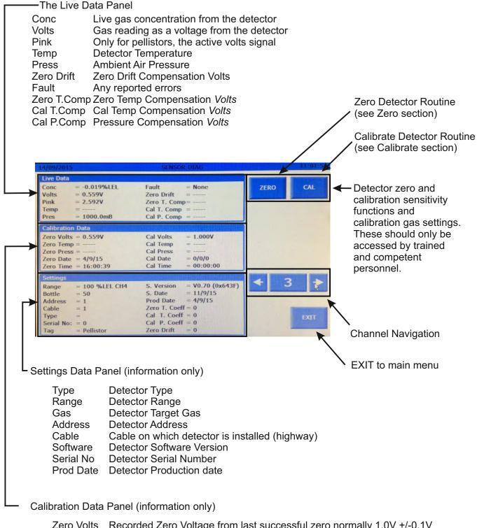
Zero Volts Recorded Zero Voltage from last successful zero normally 1.0V +/-0.1V
