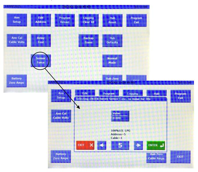
Select the channel to force and then enter the required value. With the correct channel and value displayed, selecting enter will force that level onto the selected channel for *30* seconds. This allows testing of the alarm configuration without having to use test gas or signal generators.
