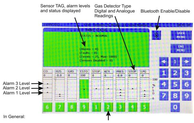
Green = Normal Red = Alarm Yellow = Fault Black = Disabled Click on a displayed channel number to make it the currently viewed channel or type in the channel number of interest. Note that the display centres on the selected channel and displays its current status
