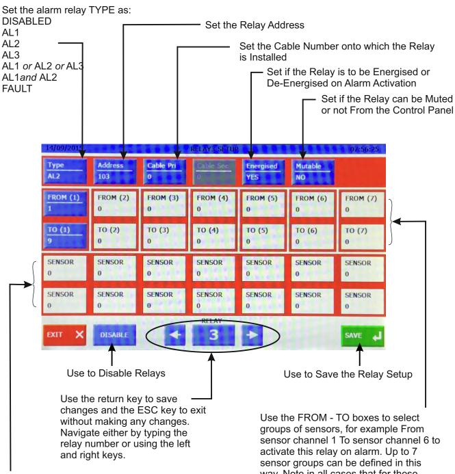
In addition to the FROM - TO sensor groups, individual channels can also be added into the relay activation definition. Up to 14 individual sensor channels can be added to the definition. Note in all cases that for these sensors channels the relay will be active only for whichever alarm level, AL1,2 or 3 is defined in the relay TYPE.
