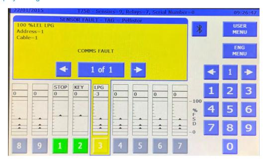
Faults are indicated on screen as a 'Yellow' display. Faults will be indicated against either the system or against the channel that has a fault. Alarms take precedence over faults but will still be indicated on screen at the side of the main display panel.
