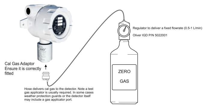
IMPORTANT: Flow gas for a minimum of 60 Seconds. Some detectors with longer response times may take longer to stabilise.
