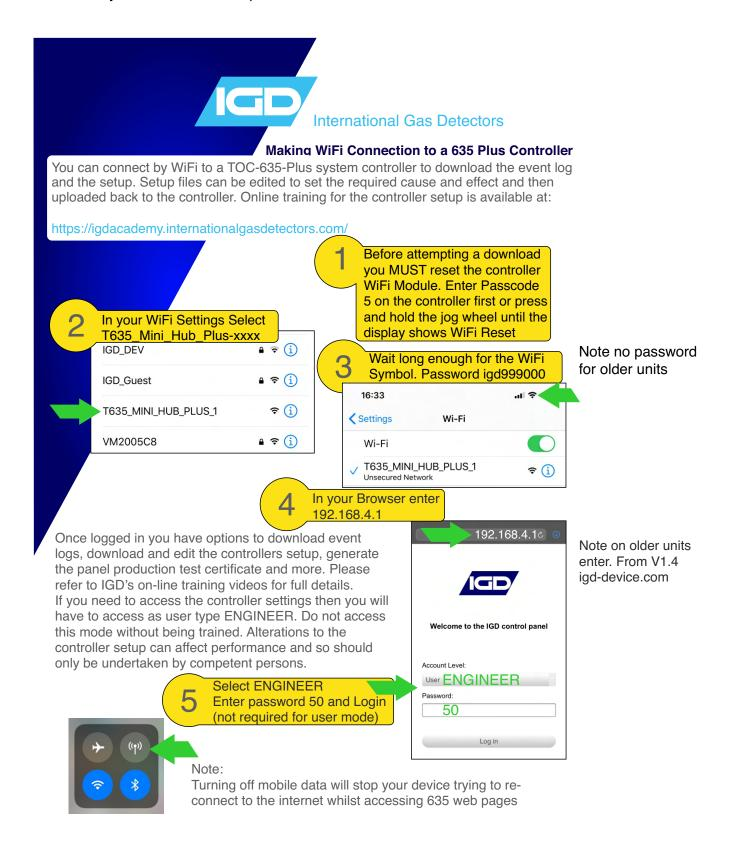
Note that whilst editing a controller setup you MUST stay within WiFi range. If you want to edit a downloaded setup offline, IGD provide a website that allows you to open, view and edit a previously downloaded and stored setup.
