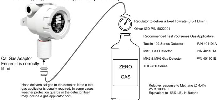
IMPORTANT: Flow gas for a minimum of 60 Seconds. Some detectors with longer response times may take longer to stabilise.
