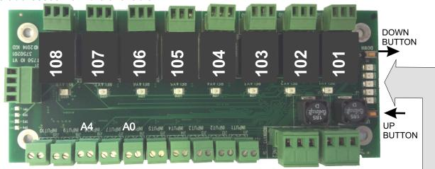
Press and hold the DOWN button until all LED's are OFF. Release the button and the address currently set will be illuminated on the bottom five LED's.
