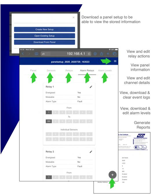
Please note that when editing your controller setup you have to stay WiFi connected to the controller. If you want to edit off-line then you must first save the panel setup. Use the enclosed QR code to access the remote web portal. You can then upload the panel setup and edit off line. Once saved you can then re-connect to the controller at a later date to upload the revised setup
