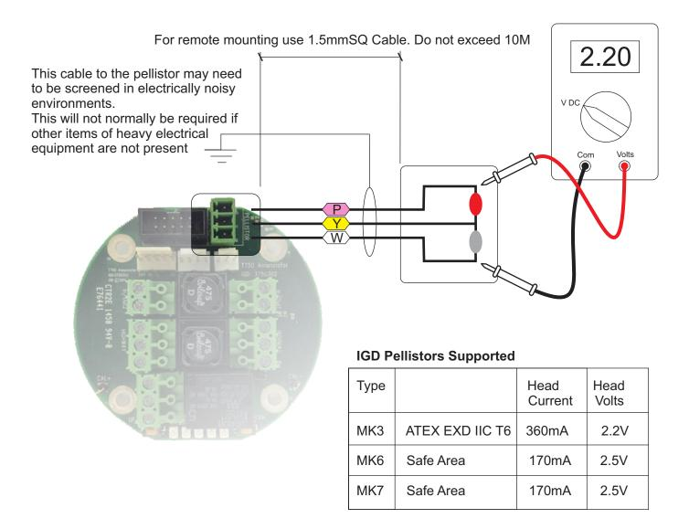
Note: The Pellistor 'Type' is selected using IGD service tool app or by using the setup routine in the TOC-750 Software. Once selected this automatically sets the head supply voltage.
