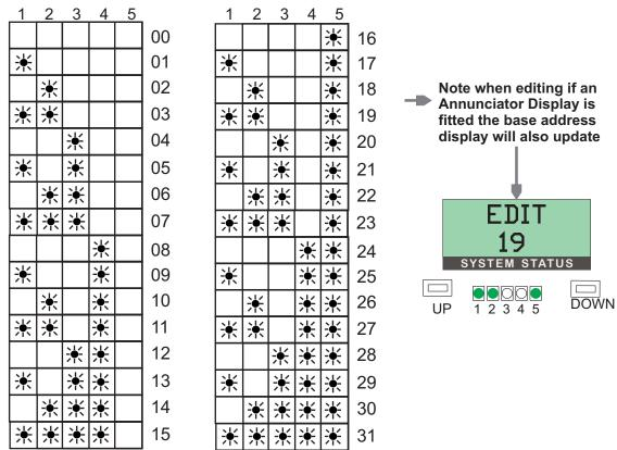
Setting the base address using the button interface sets the address for all other active options on the module as follows:
