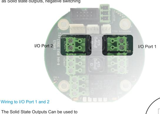
The Solid State Outputs Can be used to Switch LED Beacon Sounders if Required.
