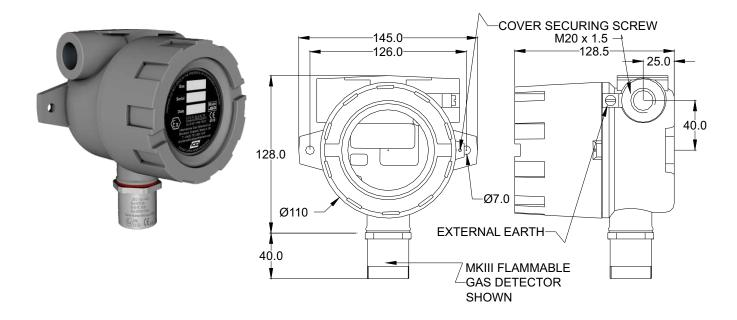
The ATEX version uses IGD's JB3 series ATEX EXD terminal enclosure. Please note that cable glanding and sealing must conform to ATEX requirements which is more fully described in the ATEX JB3 manual
