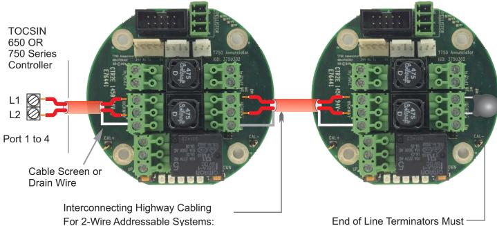
For Safe Area Detectors Use 2 Core Unscreened Cable 1.0 to 2.5mmSQ Cable Depending on Distance.
