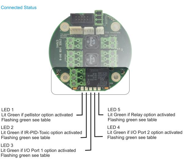
Note the LED flash rate is used to indicate as follows:
