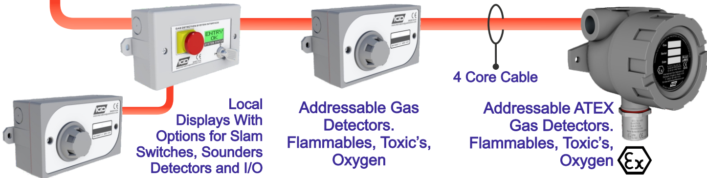
Data Highway Support up to 32 Gas Detectors/Devices Using 2 Core Cable
