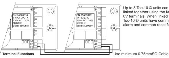
Up to 8 Toc-10 © units can be linked together using the I/O and 0V terminals. When linked the Toc-10 © units have common alarm and common reset function.
