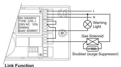
Example shows a Toc-10 © Wired to a gas supply solenoid valve and warning light. The warning light is active in this example when the first alarm level is reached (10%) and the gas solenoid is de-activated when the second alarm level is reached (25%). Note in this example a surge suppressor is fitted to the gas solenoid to extend the life of the relay. For DC solenoids a diode could be fitted. Any such installation must comply with the national regulations in force in the country EN1775 refers
