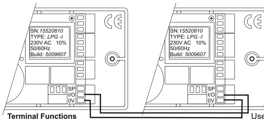
Up to 8 Toc-10 © units can be linked together using the I/O and 0V terminals. When linked the Toc-10 © units have common alarm and common reset function.
