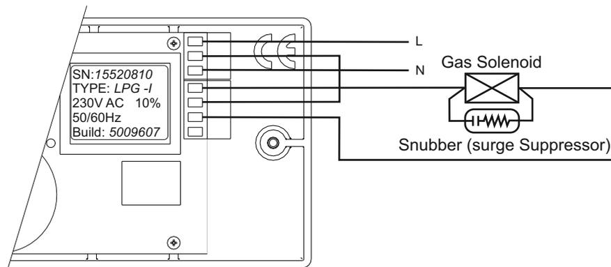
Example shows a TOC © Wired to a gas supply solenoid valve. The warning light is active in this example when the first alarm level is reached (10%) and the gas solenoid is de-activated when the second alarm level is reached (25%). Note in this example a surge suppressor is fitted to the gas solenoid to extend the life of the relay. For DC solenoids a diode could be fitted. Any such installation must comply with the national regulations in force in the country EN1775 refers
